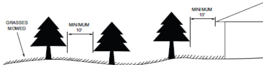
Commentary Figure 603.2.2 10-FOOT SEPARATION BETWEEN TREE CROWNS AND STRUCTURES
